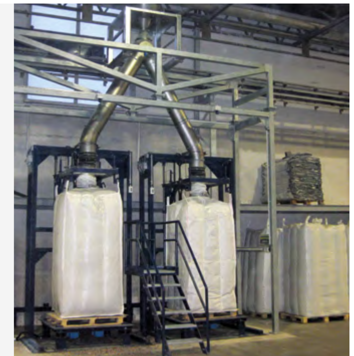
Pipe trough metering screw conveyor with spout plug valve to restrict or increase the bulk density
